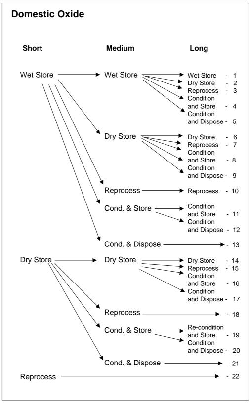
Figure 3.1. Option Diagram: Domestic Oxide Fuel
