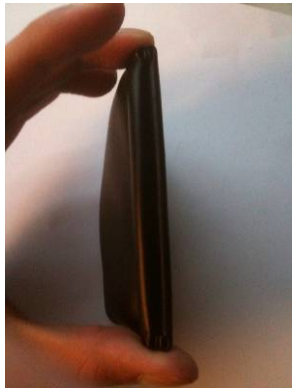
Stable equilibrium: When no force is applied the strips are straight and the pouch closed
