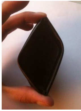
Neutral equilibrium: Gradually the force applied by the fingers is increased until sudden buckling
