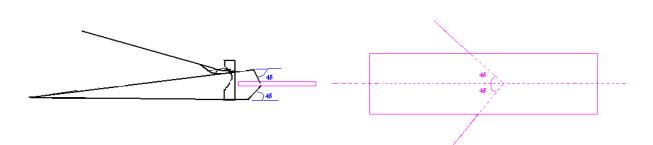
If we use nail clipper to chop the corner of one plane paper as it is shown in first picture a little force on the lever arm is sufficient to cut it. But as we locate the blades in the middle of the same paper the greater force is needed and it is because of increment in paper area subjected to the force. It is clear when we fold the paper and redo the same action greater force must be applied due to having thicker depth.
