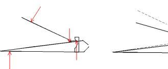
firs drawing. Once we apply the force on lateral arm, lower finger holding the clipper acting as support. Sketches show the actions and reactions forming clipper mechanism.
