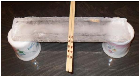
Figure 2- unreinforced ice beam(1)
