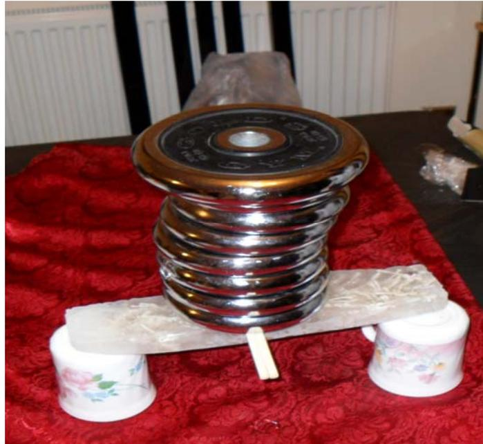
Figure 4: ice beam (2) – reinforced beam supporting a load of 11.25kg
