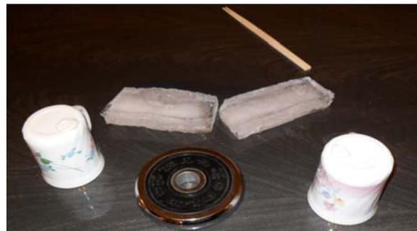
Figure 3 – Ice beam (1) failed under load of 1.25 kg
