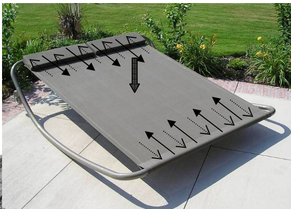
Figure 9: Rocking Hammock As any other hammock, for this portable unit to have any functionality, one must be able to lie on it whilst the hammock remains stable supporting ones mass. In order to achieve this, the fabric is tensioned (pulled) and wrapped around the metal beam at the edges. The fabric has a pre-tensioning force within; the force resulting from the mass is applied vertically, resulting in forces that act opposite to the pre-tension forces. The balance is such that the mass remains suspended on the fabric, whilst the fabric is tensioned. The pre-tensioning means that the overall resulting forces on the member are much smaller. In any case where the fabric was not pre-tensioned, the mass would sink when applied.
