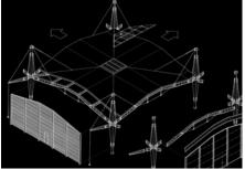
The self-balancing structure is two-directional and creates a  $24m^2$  module.
