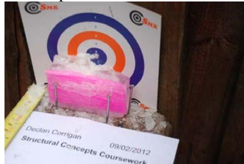
Test Five: Frozen water and plastic fibre reinforcement (18 coils)
