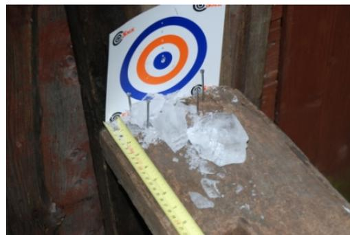
Test Two: Frozen water and steel fibre reinforcement (staples)
