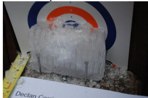
Test Four: Frozen water and plastic fibre reinforcement (20 straws)
