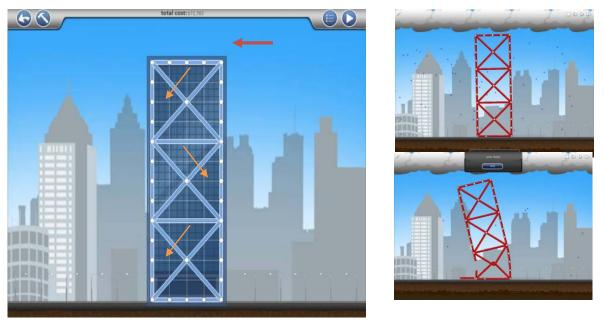
The third bracing layout fulfills all of the above criteria. The bracing flows from the top of the building to the bottom and the bracing in each adjacent level and bay are joined where possible. This is a very effecting bracing pattern, however due to the extreme force of the wind in this simulation; the building eventually fails albeit at a very high wind speed.
