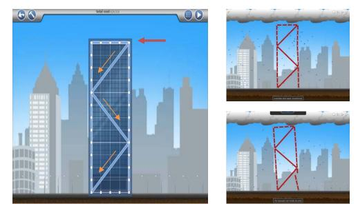
To improve the structure it is necessary to add more bracing members to improve the force path. Using a cross bracing layout, you will see that the bracing criteria are still being followed
