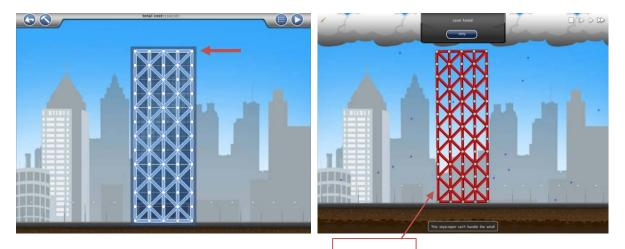
The next bracing layout shows the structure being fully braced down both sides, with adjoining bracing across the top. The cross bracing down each side provides a good direct force path to transfer the force of the wind down to the ground. The bracing layout allows the building to sway slightly but ultimately it keeps the building stiff enough to resist failure.
