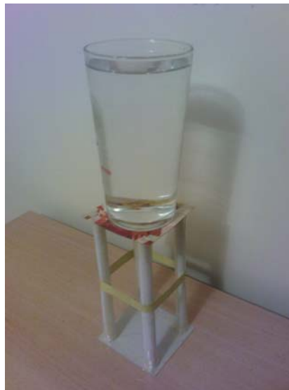
Figure 4. Improved arrangement supporting a pint of water
