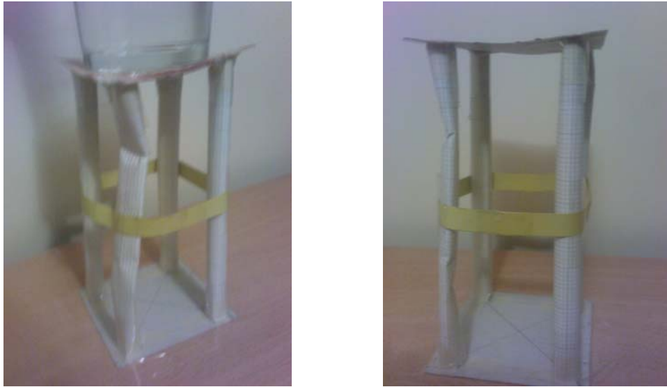
Figure 5. Failed column on improved arrangement
