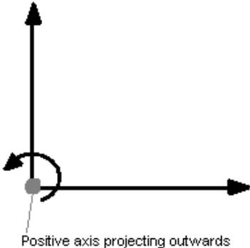
Figure 2: 2-D diagram - positive moment appears anti-clockwise
